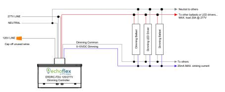
Echoflex ERDRC-FDU · Mounts through ½\* knockout into J Box or fixture · Communications on 902 MHz frequency · 0-10V dimming capability up to 25mA of sinking current · Controls up to 20A of lighting Igoad · Configurable through software or other mechanical means · Transmission range 0124 m (80 Fly up to 100 m (330 ft) line of sight)
